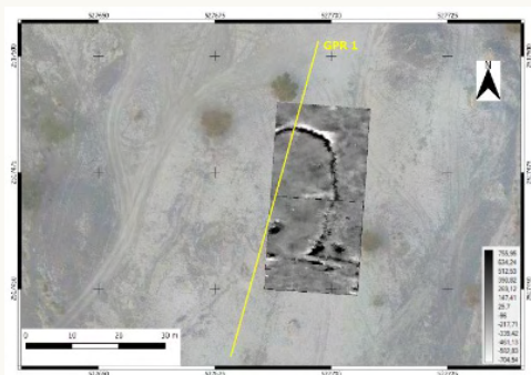
Figure 3 :Al Dhabi 5 3D geomagnetic survey showing an oval structure due to the high contrast between the dug ditch filled with brown-orange clay/silt material and the surrounding floodplain material (left). Field measurements (right).
