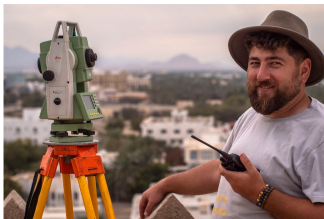
Figure 7. Topographic mapping of the town with a total station system, photogrammetry and GIS. Photo Peter Brown.
